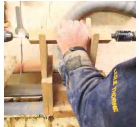
▲ Pic.3 Due to regulations, the candle can't come in direct contact with the timber. The brass candle cup requires a 22mm hole - 'V' blocks will allow you to drill an accurate hole, just wind the wood onto the spinning drill
